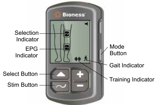
Figure 7-1: Selecting a Operating Mode on the Control Unit
