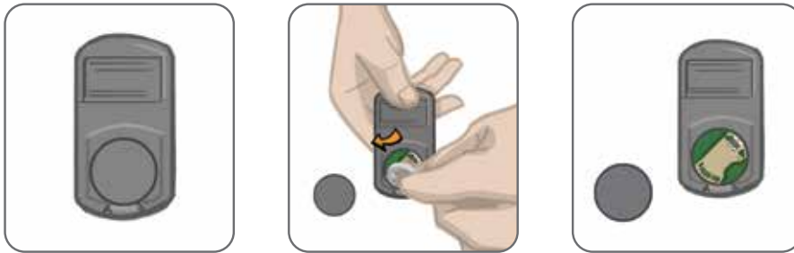
Figure 8-2: Replacing the Control Unit Battery
